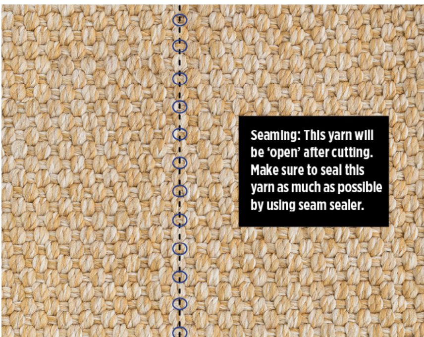
Figure 2: Take care to leave lower lockstitch on “good” side of seam
